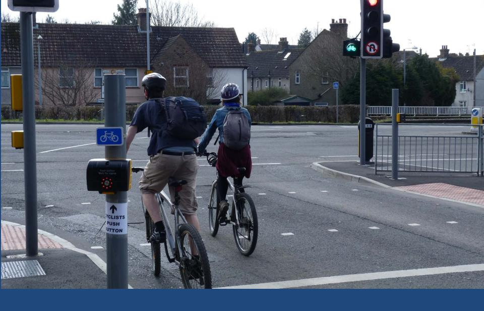
Node 01 Newly installed push-button operated advanced cycle signal allows cyclists to turn right across the A270 three seconds ahead of other traffic.
